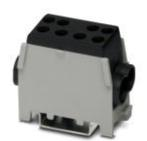
Trunk line branch terminal, nom. voltage: 400 V, nominal current: 125 A, connection method: Screw connection, Screw connection, number of connections: 4, number of positions: 1, cross section: 10 mm² - 35 mm², AWG: 8 - 2, width: 27 mm, color: black, mounting type: NS 35/7,5, NS 35/15
