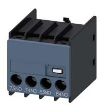
Auxiliary switch on the front, 2 NO Current path 1 NO, 1 NO Connection from below for 3RH and 3RT screw terminal 73/74, 83/84
