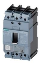
circuit breaker 3VA5 UL frame 125 3-pole, starter protection TM120M, AM, In=5A without overload protection short-circuit protection li=3...7 x In cable connection on both sides
