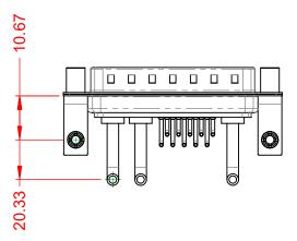
20A (CURRENT) POWER/CO-AX CONTACT RATING: (IF PRESENT) SIGNAL CONTACT CURRENT RATING: 5A PER CONTACT SIGNAL CONTACT RESISTANCE:  $10m\Omega$  MAX.
