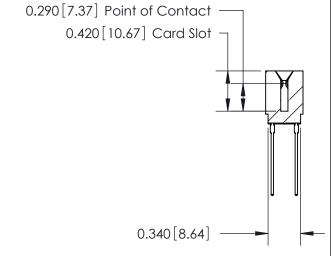
726 Series Ultra-Mate Card Edge Connector - Press Fit Part Number: 726-056-541-201
