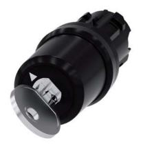
key-operated switch Siemens, 22 mm, round, plastic, lock number SSG10, with 2 keys, 2 switch positions O-I, latching, actuating angle  $90^\circ, 10:30h/13:30h,$  key removal O+I, with laser labeling, upper case
