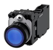
Illuminated pushbutton, 22 mm, round, plastic, blue, pushbutton, flat, momentary contact type, with holder, 1 NO+1 NC, LED module with integrated LED 24 V AC/DC, screw terminal, with laser labeling, lower case
