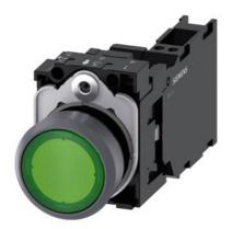
Illuminated pushbutton, 22 mm, round, plastic with metal front ring, green, pushbutton, flat, momentary contact type, with holder, 1 NO+1 NC, LED module with integrated LED 24 V AC/DC, spring-type terminal, with laser labeling, upper case and lower case, always upper case at beginning of line
