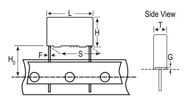
General Information Series Dielectric Metallized Polypropylene Style Radial Features MKP EMI Safety RoHS Lead Wire Leads Safety Class X1 Qualifications ENEC, UL, cUL, CQC AEC-Q200 No THB Performance No Component Weight 3.258 g Miscellaneous ClimCat: 40/110/56/B Shelf Life 104 Weeks
