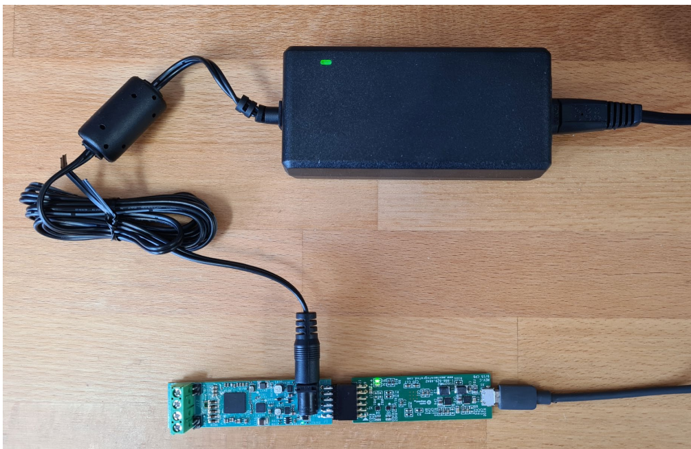
Figure 2. USB cable between the PC and the USB2PMB2#.
