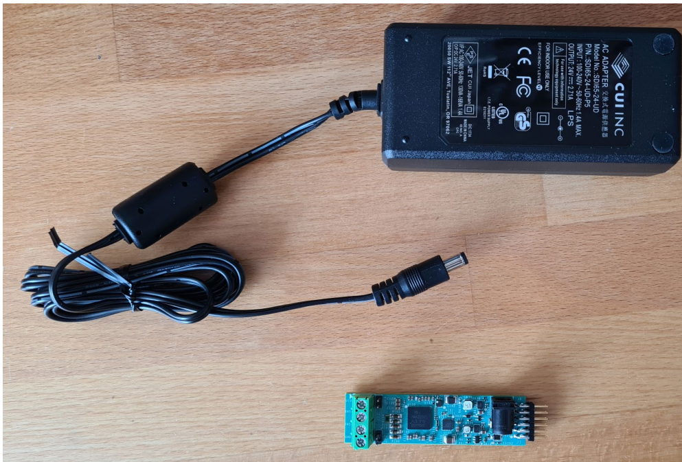
Figure 1. 24V barrel-connector supply to MAXREFDES185#.
