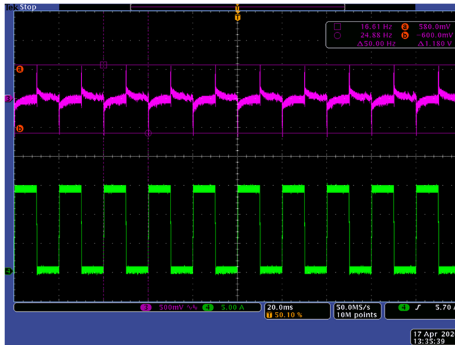
Figure 18. No Load to Full Load Transient (CH3=LLC Output AC Coupled; CH4=Output Current)
