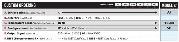
Note: Outputs are field selectable between 0-5 VDC & 0-10 VDC
