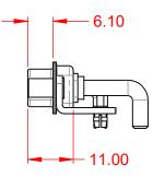
NOTES: MATERIAL: HOUSING: THERMOPLASTIC POLYESTER, UL94V-0 STEEL, TIN PLATED SHELL: COPPER ALLOY, GOLD FLASH PLATED CONTACT: **OPERATING TEMPERATURE:** -55°C ~ 125°C 40A (CURRENT) POWER/CO-AX CONTACT RATING: (IF PRESENT) SIGNAL CONTACT CURRENT RATING: 5A PER CONTACT SIGNAL CONTACT RESISTANCE:  $10m\Omega$  MAX. O
