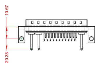
POWER/CO-AX CONTACT RATING: 10A (CURRENT) (IF PRESENT) SIGNAL CONTACT CURRENT RATING: 5A PER CONTACT SIGNAL CONTACT RESISTANCE:  $10m\Omega$  MAX. INSULATOR RESISTANCE:  $5000M\Omega$  min. DIELECTRIC
