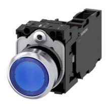
Illuminated pushbutton, 22 mm, round, metal, shiny, blue, pushbutton, flat, momentary contact type, with holder, 1 NO+1 NC, LED module with integrated LED 110 V AC, screw terminal, with laser labeling, upper case
