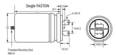
General Information Series C87 Dielectric Film/Foil Polypropylene Style Aluminum Case, Plastic Cover, Spun Seal Description Features Spun Seal, Safety Class S2, UL\_94 V0 Disk RoHS Yes Lead Fast On (1+1) UL, VDE, CQC, CSA (600VAC), UL\_94 V0 Qualifications Disk AEC-Q200 No Component 49 g Weight
