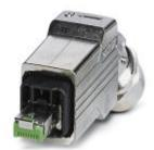
Push-pull connector (version 14), die-cast zinc, with RJ45 connector insert, 8-pos., with IDC fast connection technology, for 1 and 7-wire cores, 26 ... 24 AWG, for cable diameter of 5.5 mm ... 10 mm
