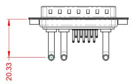
POWER/CO-AX CONTACT RATING: (IF PRESENT) SIGNAL CONTACT CURRENT RATING: 5A PER CONTACT SIGNAL CONTACT RESISTANCE:  $10m\Omega$  MAX. INSULATOR RESISTANCE: 5000MΩ min.
