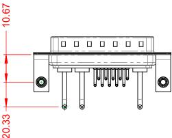
POWER/CO-AX CONTACT RATING: (IF PRESENT) SIGNAL CONTACT CURRENT RATING: 5A PER CONTACT SIGNAL CONTACT RESISTANCE:  $10m\Omega$  MAX.
