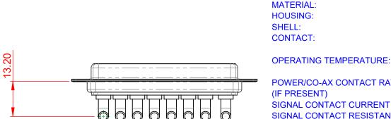
THERMOPLASTIC POLYESTER, UL94V-0 STEEL, NICKEL PLATED COPPER ALLOY, GOLD FLASH PLATED
