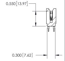
745 Series Ultra-Mate Card Edge Connector - Press Fit Part Number: 745-074-560-206
