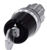
key-operated switch Siemens, 22 mm, round, metal, shiny, lock no. STGH10, with 2 keys, 3 switch positions I-O<II, left latching, momentary contact type on the right, actuating angle 2x45°, 10:30h/12h/13:30h, key removal O+I, with laser labeling, upper case and lower case, always upper case at the beginning of the word
