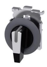
Selector switch, illuminable, 30 mm, round, Metal, matte, white, selector switch, long, front ring for flush installation, 3 switch positions I-O-II, latching, actuating angle 2x45°, 10:30h/12h/13:30h, Z=50-unit packaging
