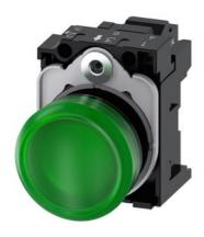
Indicator lights, 22 mm, round, plastic, green, lens, smooth, with holder, LED module, with integrated LED 24 V AC/DC, spring-type terminal, with laser labeling, inscription or symbol Customer-specific selection with SIRIUS ACT configurator (CIN)
