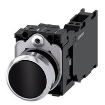
Pushbutton, 22 mm, round, metal, shiny, black, pushbutton, flat, momentary contact type, 1 NO+1 NC, spring-type terminal, with laser labeling, upper case and lower case, always upper case at beginning of line
