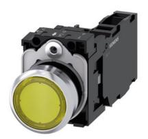
Illuminated pushbutton, 22 mm, round, metal, shiny, yellow, pushbutton, flat, momentary contact type, with holder, 1 NO+1 NC, LED module with integrated LED 24 V AC/DC, screw terminal, with laser labeling, upper case and lower case, Always upper case at the beginning of the word
