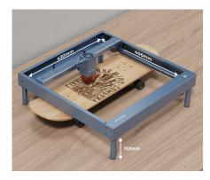
Ample working area of 430\*400mm to carry out batch processing in one go and additional risers to support thicker objects and special attachments.
