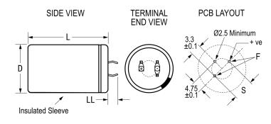
**General Information** Series PEH536 Dielectric Aluminum Electrolytic Description Snap-In, Aluminum Electrolytic RoHS Yes Lead 3 Pin Short AEC-Q200 No **Component Weight** 85 g Notes Add 0.5mm To D And 1mm To L For Sleeving. Shelf Life 208 Weeks
