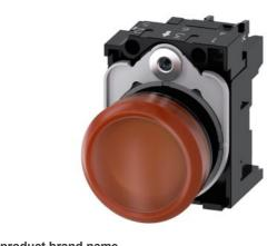
Indicator lights, 22 mm, round, plastic, amber, lens, smooth, with holder, LED module, with integrated LED 230 V AC, screw terminal
