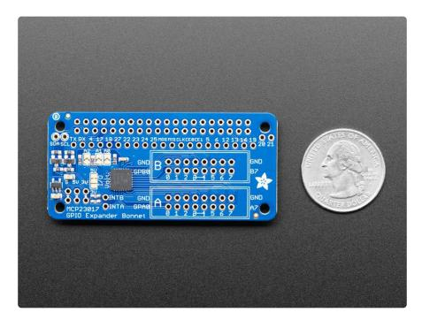
By soldering closed the address select jumpers, you can change the address from 0x20 up to 0x27. So, if you wanted to, you could have up to 8 bonnets for 128 total GPIO.
