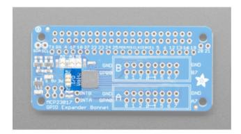
This Bonnet defaults to using 5V. There is a jumper to swap between 3V and 5V. If you want to change it to 3V, you can cut the trace between the top two pads, and solder the bottom two pads.
