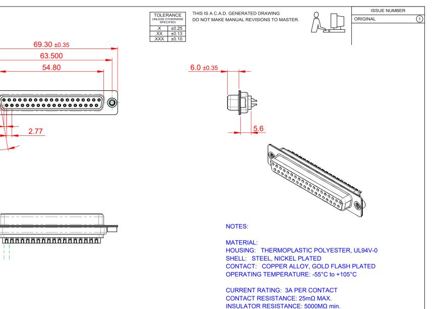
DIELECTRIC WITHSTANDING VOLTAGE: 1000V AC rms
