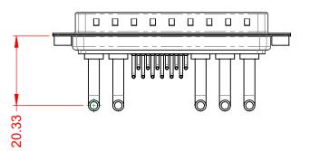
30A (CURRENT) POWER/CO-AX CONTACT RATING: (IF PRESENT) SIGNAL CONTACT CURRENT RATING: 5A PER CONTACT SIGNAL CONTACT RESISTANCE:  $10m\Omega$  MAX. **INSULATOR RESISTANCE:** 5000MΩ min. DIELECTRIC
