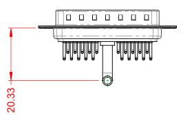
40A (CURRENT) POWER/CO-AX CONTACT RATING: (IF PRESENT) SIGNAL CONTACT CURRENT RATING: 5A PER CONTACT SIGNAL CONTACT RESISTANCE:  $10m\Omega$  MAX. INSULATOR RESISTANCE:
