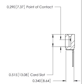
746 Series Ultra-Mate Card Edge Connector - Press Fit Part Number: 746-023-553-101
