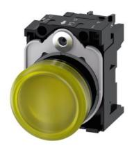
Indicator lights, 22 mm, round, plastic, yellow, lens, smooth, with holder, LED module with integrated LED 110 V AC, screw terminal, with laser labeling, symbol number according to, ISO 7000 or IEC 60417
