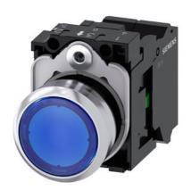
Illuminated pushbutton, 22 mm, round, Metal, shiny, blue, pushbutton, flat, momentary contact type, with holder, 1NO, LED module with integrated LED 230 V AC, spring-type terminal, with laser labeling, lower case
