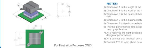
1) Dimension A is the length of the heat sink in the direction of the flow.
