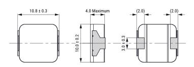
**General Information** Series MPXV Style SMD Chip Size 1040(4340) Description Surface Mount Inductor Features Power Inductors RoHS Yes Qualifications AEC-Q200 AEC-Q200 Yes Core Composite Miscellaneous 40 (K) Temperature Rise Max.
