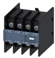
Auxiliary switch on the front, 2 NO + 2 NC Current path 1 NC, 1 NC, 1 NO, 1 NO for 3RH and 3RT Ring cable lug connection .1/.2, .1/.2, .3/.4, .3/.4
