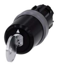
key-operated switch Siemens, 22 mm, round, plastic with metal front ring, lock number SSG10, with 2 keys, 3 switch positions I-O-II, latching, actuating angle  $2x45^{\circ}$ , 10:30h/12h/13:30h, key removal O, with laser labeling, upper case and lower case, always upper case at the beginning of the word
