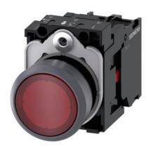
Illuminated pushbutton, 22 mm, round, plastic with metal front ring, red, pushbutton, flat, momentary contact type, with holder, 1NC, LED module with integrated LED 230 V AC, screw terminal, with laser labeling, symbol number according to, ISO 7000 or IEC 60417
