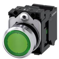
Illuminated pushbutton, 22 mm, round, metal, shiny, green, pushbutton, flat, momentary contact type, with holder, 1NO, LED module with integrated LED 110 V AC, spring-type terminal, with laser labeling, upper case
