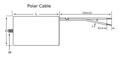
General Information Series C28 Dielectric Film/Foil Polypropylene Style Plastic Case and Cover, Ultra Sonically Welded Description Ultra Sonically Welded Seal, Safety Class S3, UL\_94 V0 Disk **Features** RoHS Yes Termination Tin Copper Lead Cables UL, VDE, UL (Construction Only), UL\_94 VO Disk Qualifications AEC-Q200 Component 38.87 g Weight
