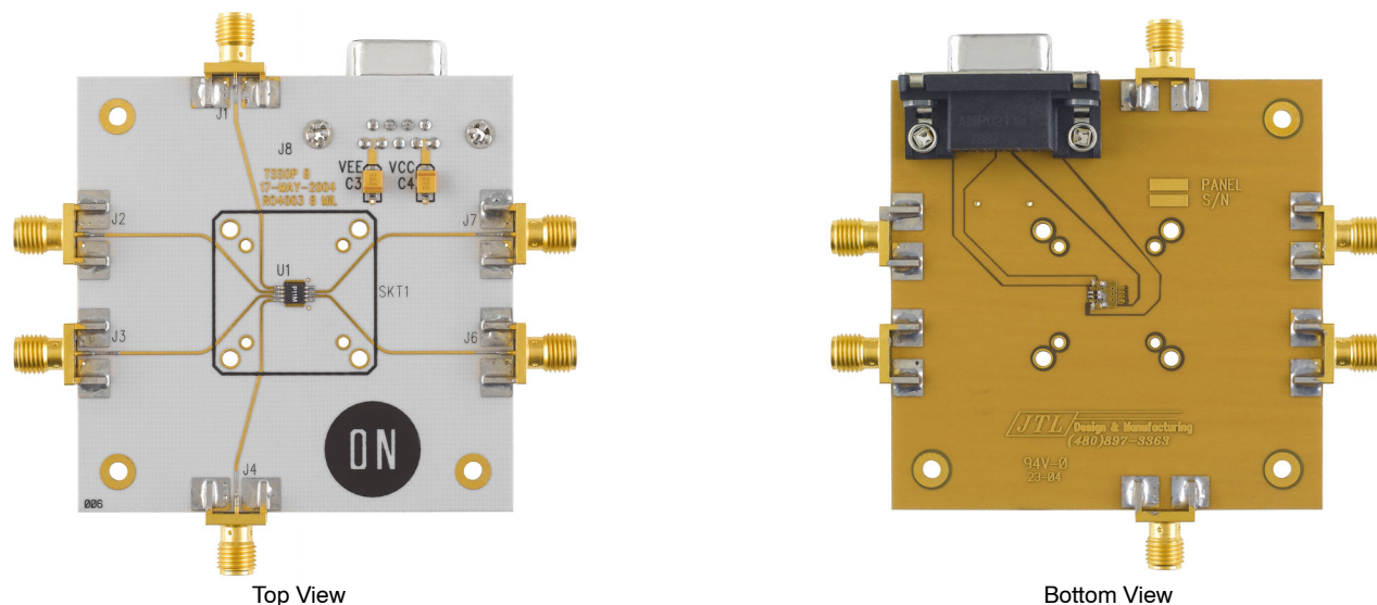
Figure 1. Top and Bottom View of the NB4N11M Evaluation Board
