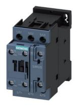
power contactor, AC-3 17 A, 7.5 kW / 400 V 1 NO + 1 NC, 400 V AC, 50 Hz 3-pole, Size S0 screw terminal
