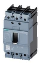
circuit breaker 3VA5 UL frame 125 breaking capacity class H 65kA @ 480 V 3-pole, line protection TM210, FTFM, In=90A overload protection Ir=90A fixed short-circuit protection Ii=10 x In UL489 SB (naval), 50 deg. cel. cable connection on both sides
