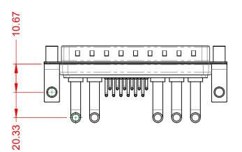
**OPERATING TEMPERATURE:** -55°C ~ 125°C 40A (CURRENT) POWER/CO-AX CONTACT RATING: (IF PRESENT) SIGNAL CONTACT CURRENT RATING: 5A PER CONTACT SIGNAL CONTACT RESISTANCE:  $10m\Omega$  MAX. **INSULATOR RESISTANCE:** 5000MΩ min.
