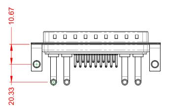
**OPERATING TEMPERATURE:** -55°C ~ 125°C 30A (CURRENT) POWER/CO-AX CONTACT RATING: (IF PRESENT) SIGNAL CONTACT CURRENT RATING: 5A PER CONTACT SIGNAL CONTACT RESISTANCE:  $10m\Omega$  MAX. **INSULATOR RESISTANCE:** 5000MΩ min. DIELECTRIC
