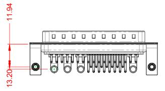
**POWER/CO-AX CONTACT RATING:** (IF PRESENT) SIGNAL CONTACT CURRENT RATING: 5A PER CONTACT SIGNAL CONTACT RESISTANCE:  $10m\Omega$  MAX. **INSULATOR RESISTANCE:** 5000MΩ min.
