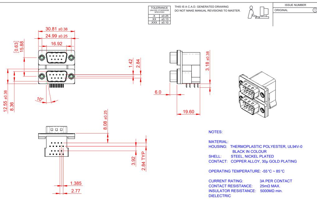
WITHSTANDING VOLTAGE: 1000V AC rms
